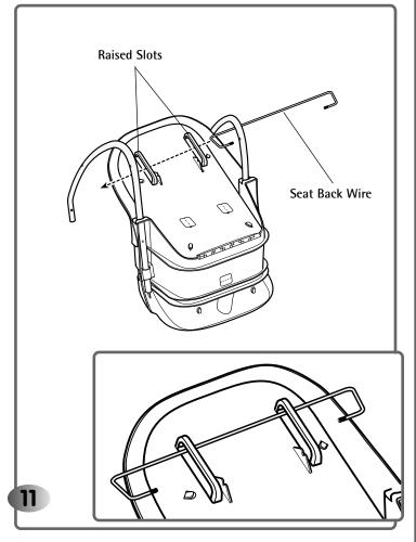
• Fit the seat back wire through the raised slots on the seat back.
